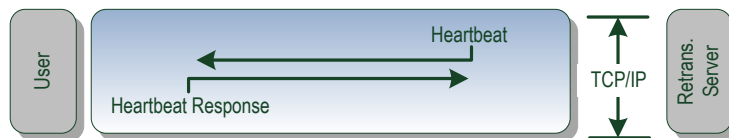
Figure 7: Retransmission Server Heartbeat Message
